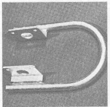
Manufactured from high-strength steel tubing and formed brackets. Prevents forks from twisting in rough terrain. Large radius allows ample clearance for oversize tires. Finished in cadmium plate. Bolts onto stock forks with no alterations required. Fits all Hodaka motorcycles.
