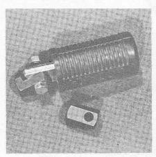
Rubber-covered folding pegs designed to be welded onto mount. Heavy-duty construction will withstand rough use of demanding competition.
