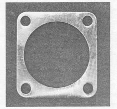
Aluminum head gaskets for 50mm cylinder bores. Eliminates having to trim out stock gasket when reboring 90cc cylinders.\* Correct thickness for proper piston to head clearance.
