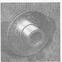
Fits all Hodaka motorcycles—replaces speedometer drive unit where speedo is removed for racing. Eliminates slight power loss from drive unit. Fabricated steel collar adds distinctive custom touch to front hub.
