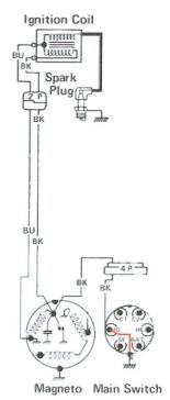
Here is the "Ignition Only" wiring diagram for the toaster tank Wombat (Model 94) . . . which almost exactly the same as for the Road Toad. The difference is that the Road Toad has a "Kill Switch" which wasn't on the Wombat.
